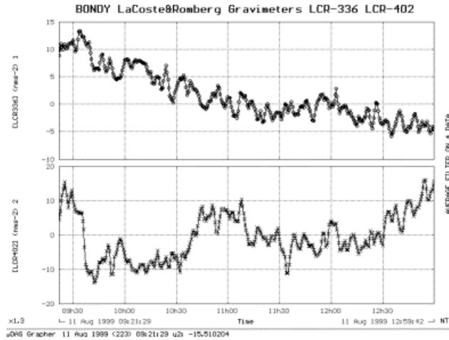
Fig. 6. Gravity changes from 9:21 to 13:00 on August 11, 1999 at Bondy station. The two curves show the de-tided records of gravity changes for the gravimeters LaCoste & Romberg 336 (top) and LaCoste & Romberg 402 (bottom). The first and last contacts at Bondy station are about 9:00 h and 12:00 h respectively, with totality at 10:30 h.
